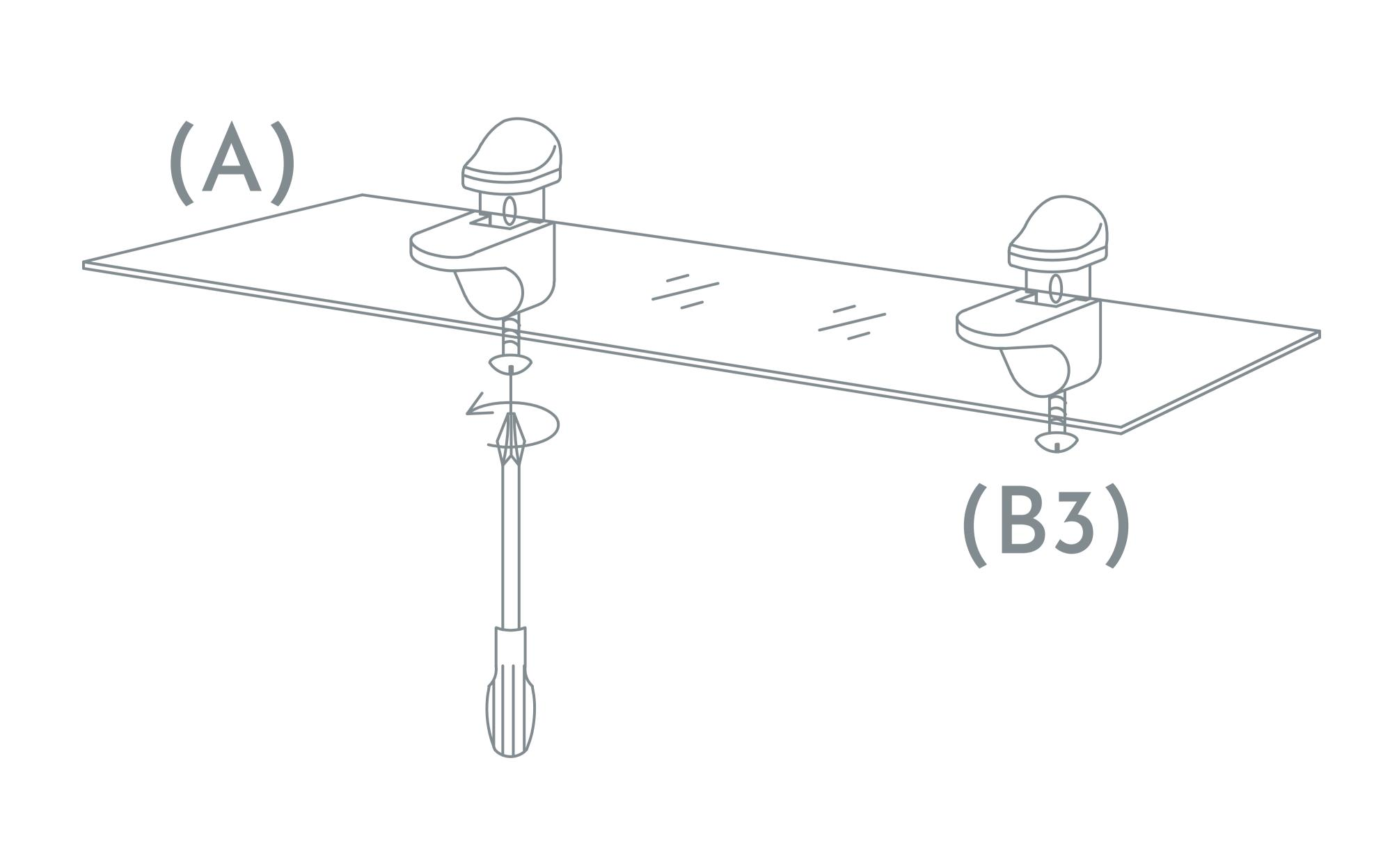
Slide Glass Shelf (A) into place and tighten Set Screw (B3). That's it!
