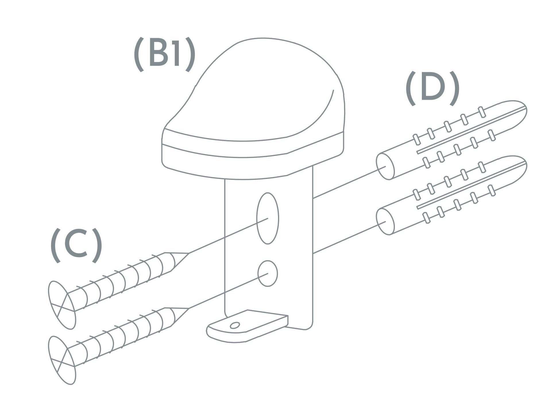
Drill pilot holes into wall for each bracket. Approximately 12" between brackets. Tap Anchors (D) into wall. Attach Upper Half (B1) of bracket to the wall using the included Screws (C).
