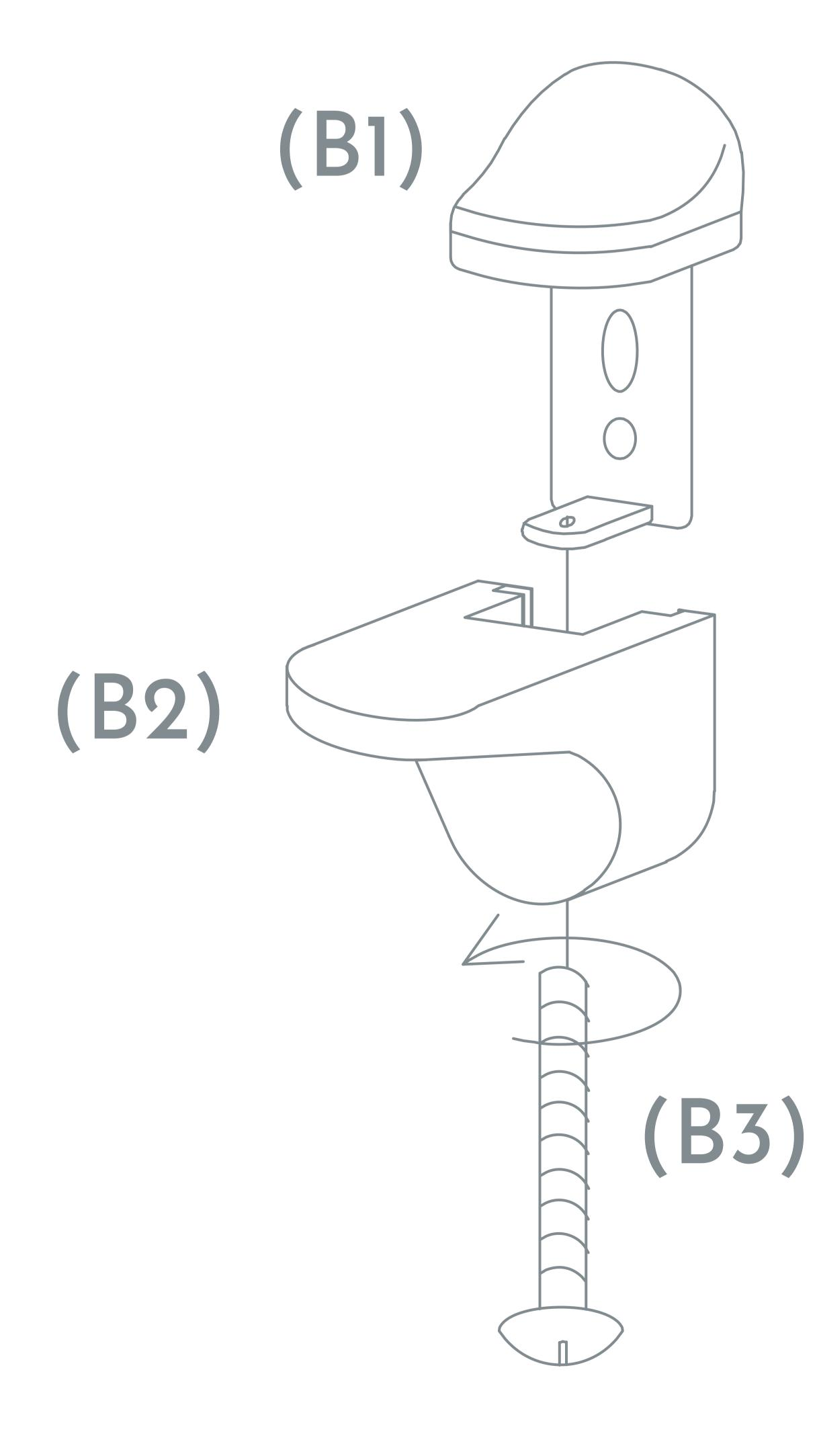
Partially attach the Lower Half (B2) bracket to the Upper Half (B1) bracket using the Set Screw (B3).
