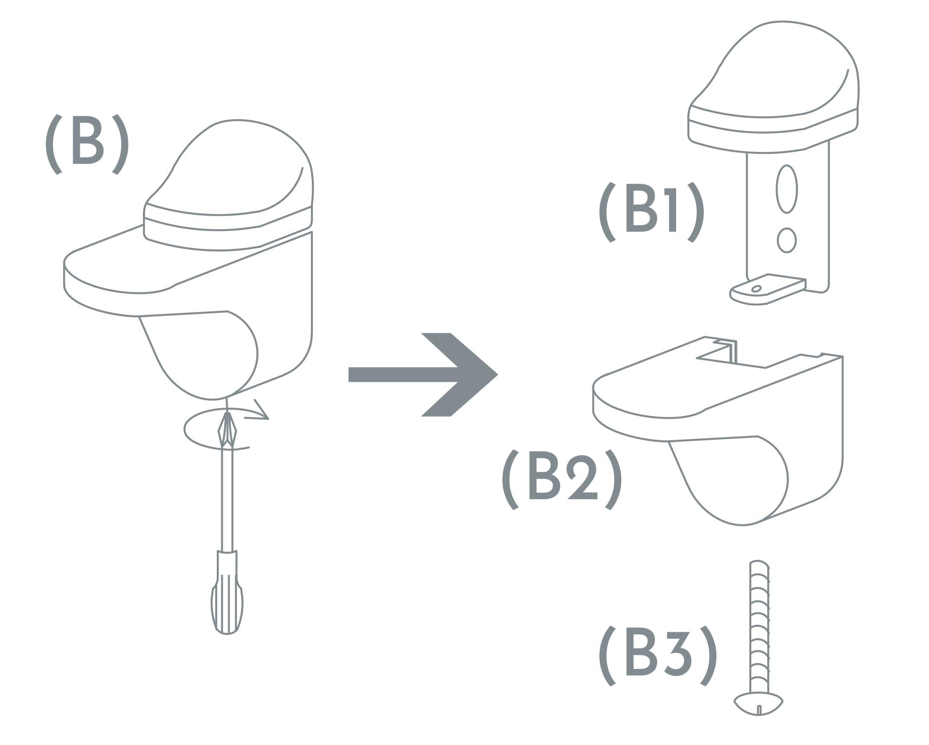
Separate each Bracket (B) into 3 parts by removing the Set Screw (B3) on the bottom of the Bracket. You will now have an Upper Half (B1), Lower Half (B2), and the Set Screw (B3).
