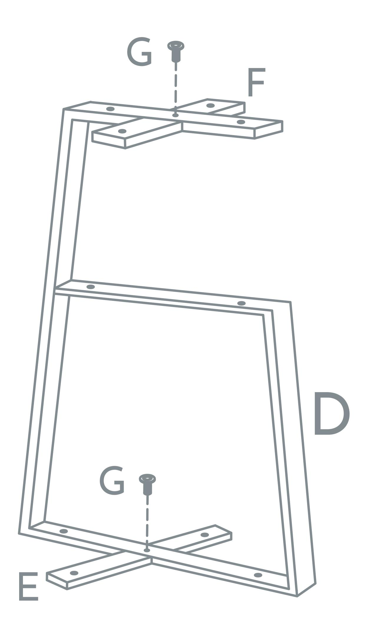
Use the Hex Key (J) and Screws (G) to fasten the Bases (E and F) (H) to fasten the Surfaces (A, B, to the the bottom and top of the Frame (D) respectively.
